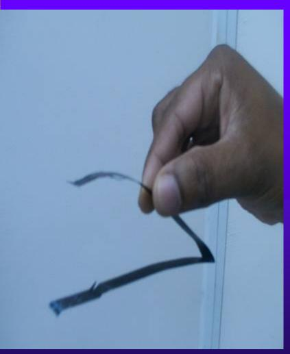
• The trap is made up of XRAY film, which is the preferred material by thieves; Simply because of the black color which is similar in appearance to the slot on the card reader.
