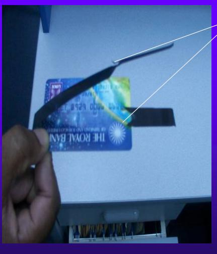
Slits are cut into both sides of the trap, This prevents your card being returned prior to completing your transaction.
