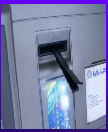
• The trap is then inserted into the ATM slot. Care is taken not to insert the entire film into the slot, the ends are folded and contain glue strips for better adhesion to the inner and outer surface of the slots.
